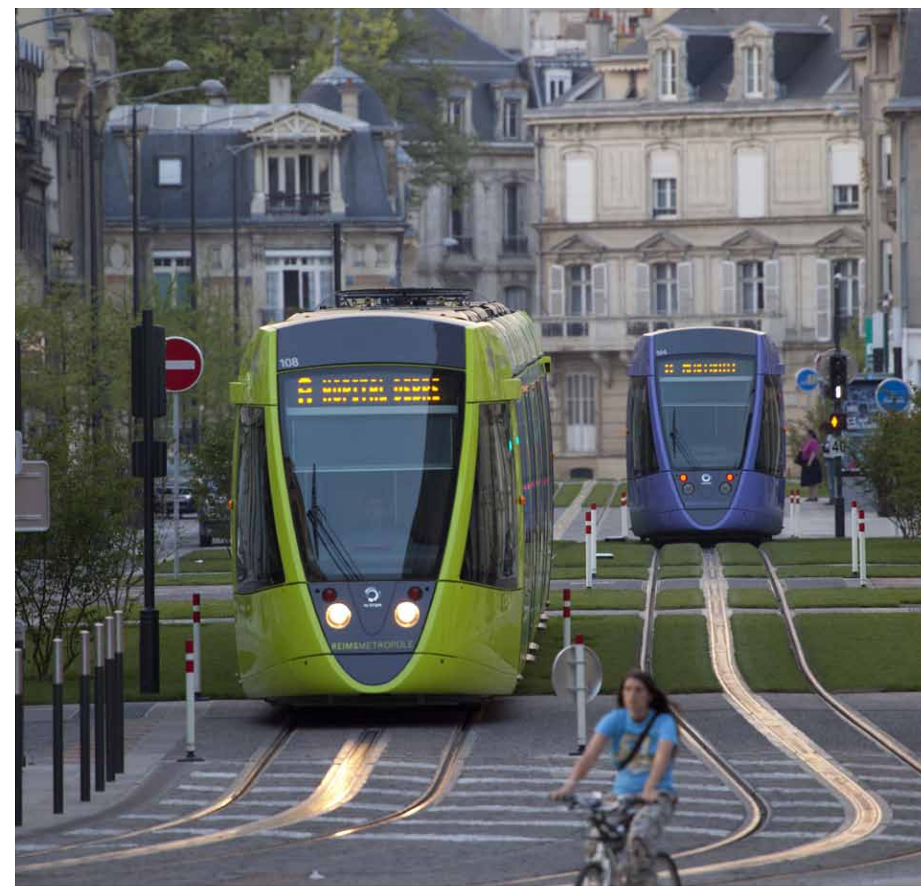
Reims, France - Aesthetic Power Supply (APS).
